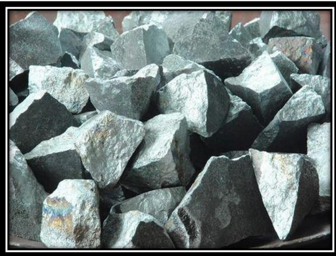
**Silico Manganese is an essential component as an ingredient in the process of manufacturing various grades of steels. Silico Manganese, High Carbon Ferro Manganese, Medium Carbon Ferro Manganese, is covered under routine production planning. In addition the existing EAF has also successfully produced Pig Iron on market demand.**
